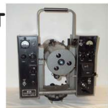
ALSA 2006.24.01 Geodimeter Model 6 introduced in 1964
